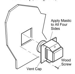
Figure 13 - Installing Horizontal Vent Cap
